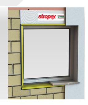
Thermo-PROFILE with transport feature is a modern product being part of all STROPEX EMO systems and it a basic component of profile system. It is made of PVC plastics filled with hard closed cell polyurethane foam with gasket and due to special shaping of the profile allows executing correct, tight and warm connection during installation of window joinery.
