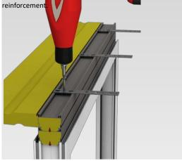
Installation of thermo-windowsill and thermo-profile should be started with the installation of the thermo-profile in the window frame. Specially designed lock, so-called click, allows correct setting of thermo-profile in the window frame (precise setting of the profile in accordance with the window geometry). Specially designed gasket allows executing tight, maintenance-free connection of profile with the window frame.
